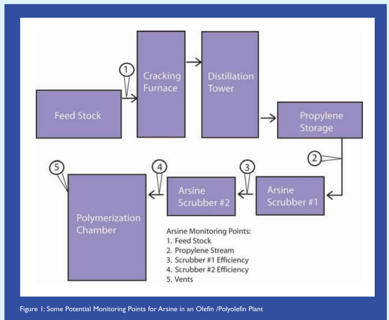
Figure 1: Some Potential Monitoring Points for Arsine in an Olefin /Polyolefin Plant
