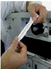
hydrocarbons) is introduced to the reaction tube where it is converted to Hydrogen sulphide ( $H_2S$ ). This gaseous sample reacts with the specific  $H_2S$  Sensi-Tape and as a result a chemical reaction happens on the paper leading to a visible stain. As clearly indicated by ASTM method D4045 the concentration of  $H_2S$  measured by this method excludes all interference from other sources which is extremely important during the analyses of complex hydrocarbons mixture.
